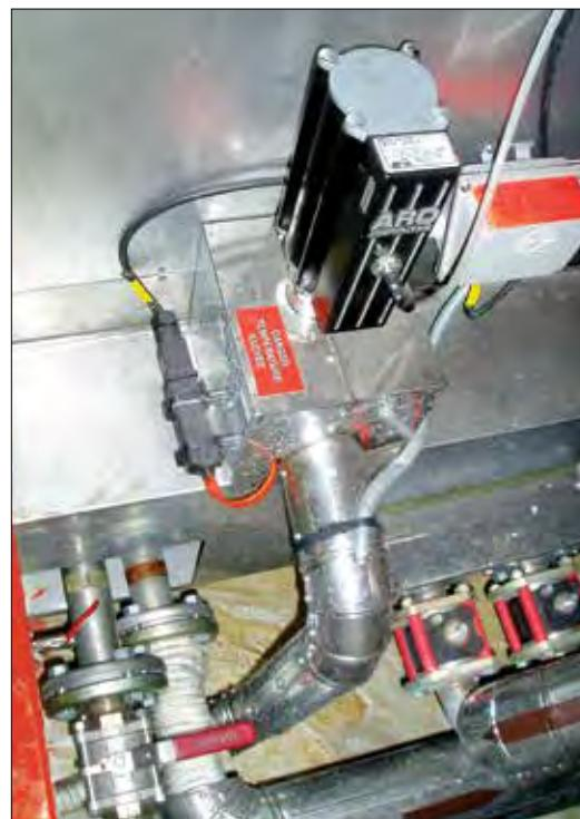
Patented ARO® Stall-Free, Ice-Free Air Motor Design: Your guarantee of trouble-free pump operation. The N Series air motor contains fewer parts and requires absolutely no mechanical assist devices such as trip rods or push pins.
